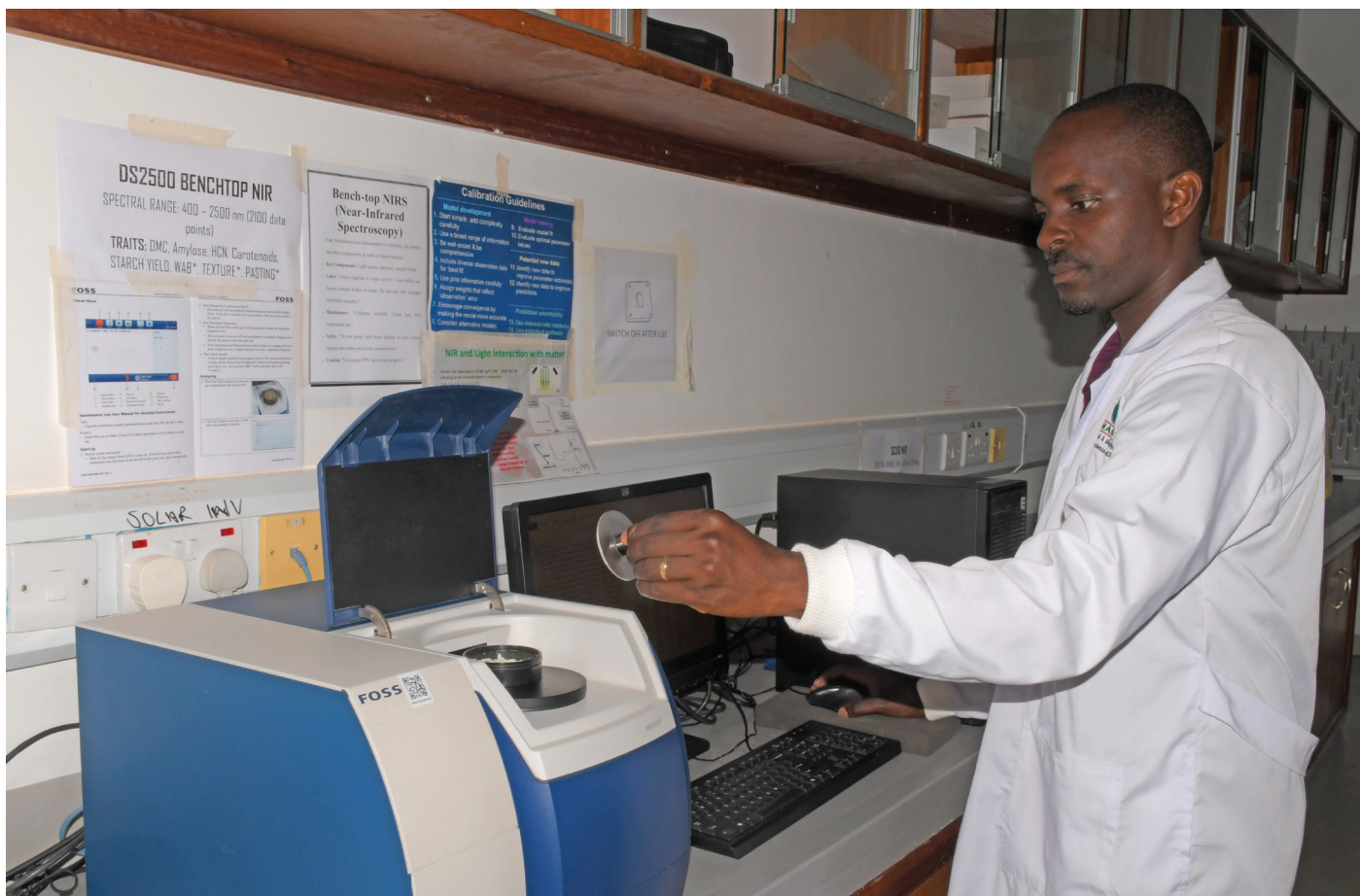
Enoch Wembabazi- Biochemist analysing a cassava sample under infrared light to measure its starch content.
