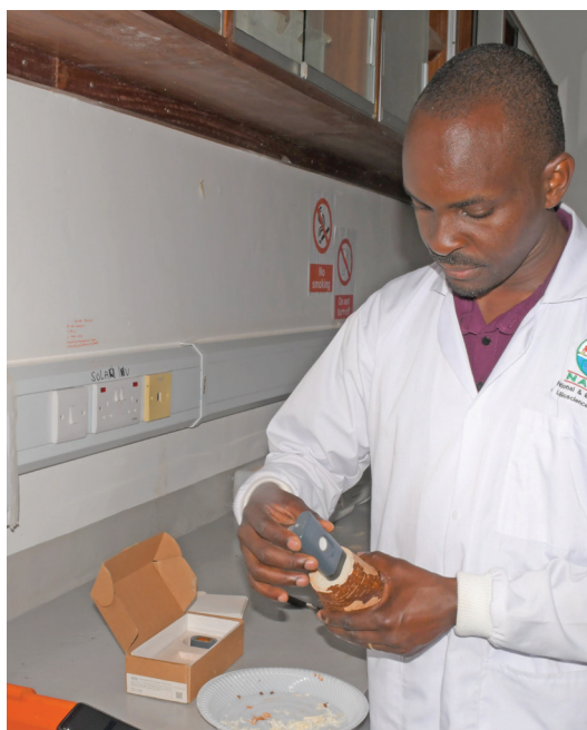
A cassava sample is being analysed and processed using a mobile application connected to an infrared light source. January-June 2025
