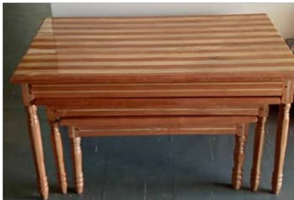
Timber offcuts glued together using resin glue
